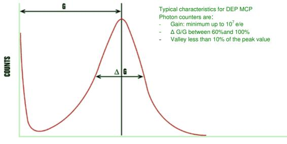
**PULSE HEIGHT/GAIN** <u>Figure 13</u>. Saturated Pulse Height Distribution for MCP photon counters
