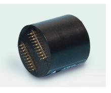
camera electronics produces a monochrome composite video signal that can be viewed on a monitor. The compact ICCD package makes sure that low light level cameras are lightweight and compact. This can be a vital detail in surveillance and security situations.
