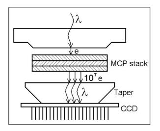
Figure 14. MCP amplifier with CCD read-out
