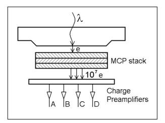
Figure 15. Resistive anode intensifier
