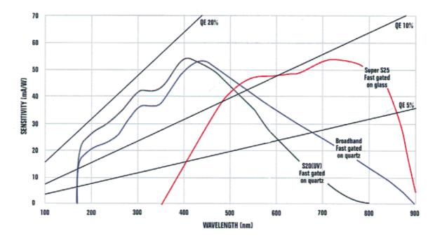
Figure 11. Photocathode types (fast gated)
