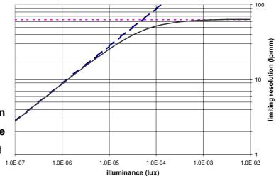
Figure 1. The limiting resolution as a function of illuminance showing the high and low light level regimes
